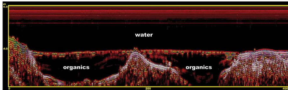
Figure 18: GPR output for a freshwater lake with thick organic materials. Water, mineral soil materials, and organic soil materials are easy to identify from the output.
