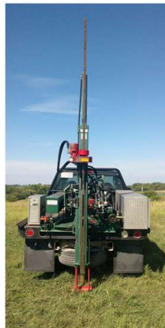
Figure 1: A truck-mounted hydraulic probe used to quickly obtain soil profiles.
